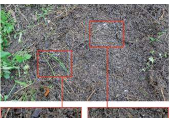
After 60 days only minimal traces in the form of silver spots remained visible. Magnification of the red fields shows the remaining traces of the original four wrapper foils. If the compost heap had been prepared professionally, no more traces would have been visible. Homecompostability was able to be demonstrated under the most basic of conditions.
